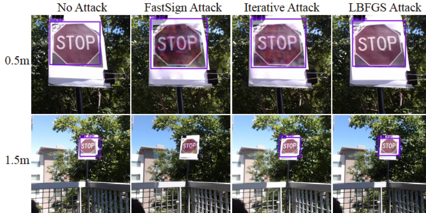
Figure 3: This figure shows experiment setup, and we use the printed stop signs to simulate real stop signs with natural background. These are examples for successful 0.5 meters and 1.5 meters detection: both original images and adversarial examples are detected in both distances. It demonstrates that adversarial examples in a physical setting do not reliably fool stop sign detectors.
