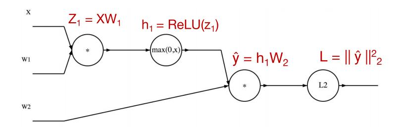
Forward pass: solve for z<sub>1</sub>, h<sub>1</sub>, ŷ and L
